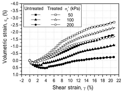
(b) Volumetric Strain – shear strain relations
