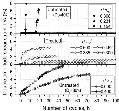
Figure 9. Developments of shear strain during cyclic loading.
