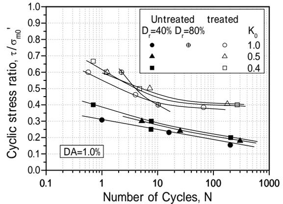
Figure 10. Reduction of the cyclic stress ratio with increasing the number of cycles.
