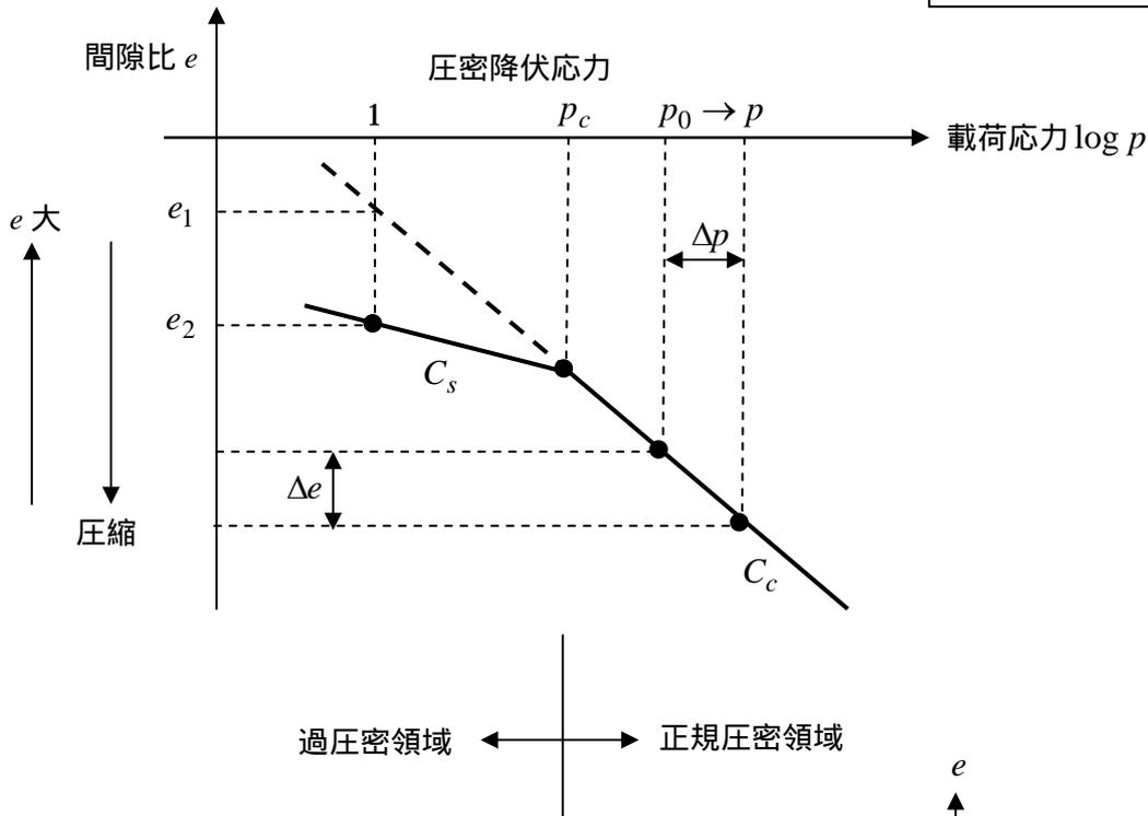
$\left\{ \begin{array}{l} p \geq p_c \text{ (正規圧密領域)} \\ e = e_1 - C_c \log p \\ p < p_c \text{ (過圧密領域)} \\ e = e_2 - C_s \log p \end{array} \right.$
